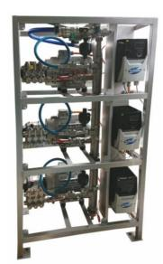
Its features make it suitable for use in process manufacturing plants, fishing vessels, aquaculture and industry in general. Connections should be made with flexible hoses to reduce noise. The high-pressure washer is supplied with vibration dampers between all three pumps and frame.
